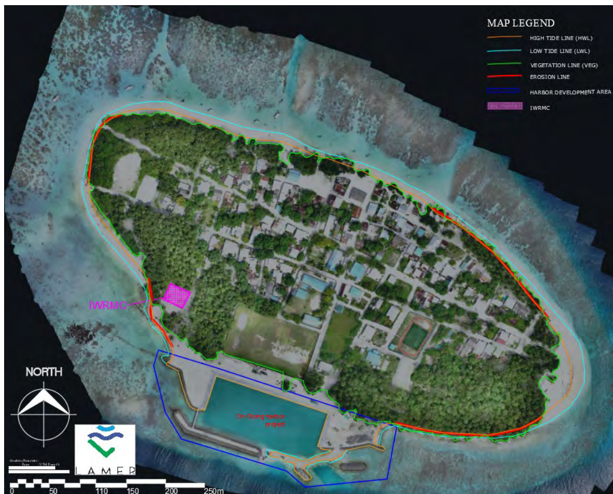
Figure 9. Erosion prone areas of Dh. Rinbudhoo (red outline) (large scale map given in Appendix 4)
