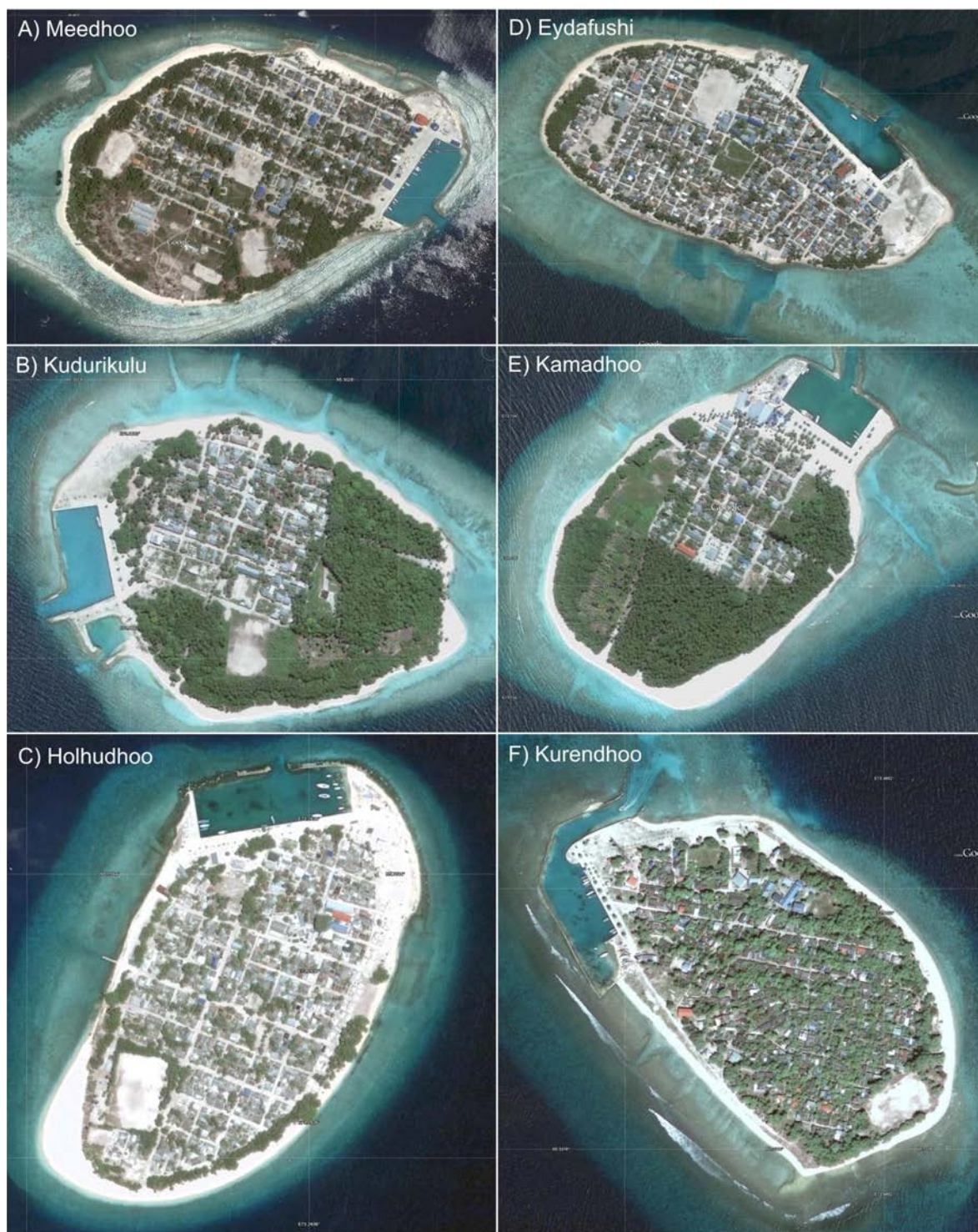
Figure 4.2. Aerial photographs of six atoll islands showing the location and configuration of boat harbours. Note physical structures and dredged areas (harbour basins and channels). Source: Google images.
