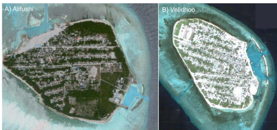
Figure 4.3. Aerial photographs of two atoll islands showing the location and configuration of boat harbours with disconnected breakwaters allowing greater alongshore flow. Source: Google images.
