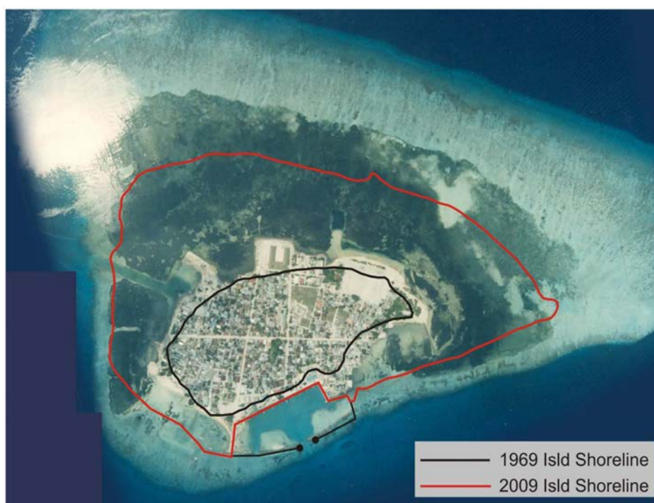
Figure 4.4. Changes in planform configuration of Naifaru (Lhaviyani) 1969 to 2009. The 1969 and 2009 shorelines are projected on the 1998 aerial photograph. Note the rapid expansion in island area between 1998 and 2009 as a consequence of dredging and reclamation.
