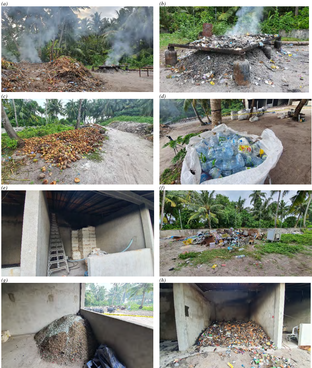
Figure 8. Waste segregation at F. Nilandhoo IWRMC. (a) Mixed waste and ash residues, (b) open burning, (c) green waste (coconut husks), (d) plastic waste in jumbo bags, (e) regiform boxes, (f) metal or bulky waste, (g) crushed glass and (h) metal cans
