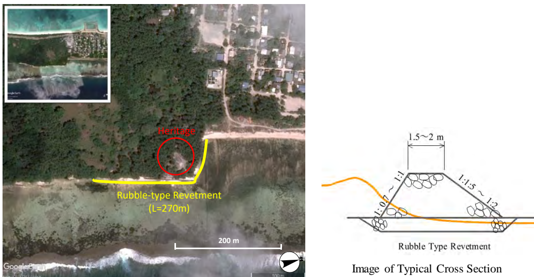
Figure 8.3.7 Coastal Protection Measure at Gan Island in Laamu Atoll
