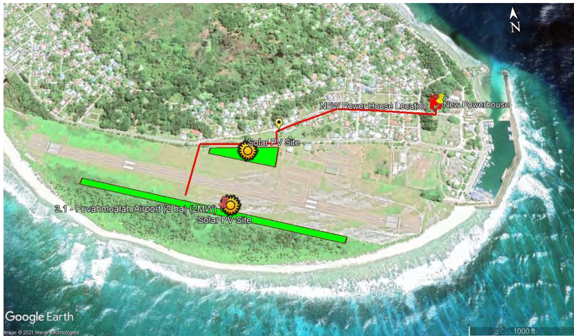
FIGURE 5 SOLAR PV GRID CONNECTION DETAILS
