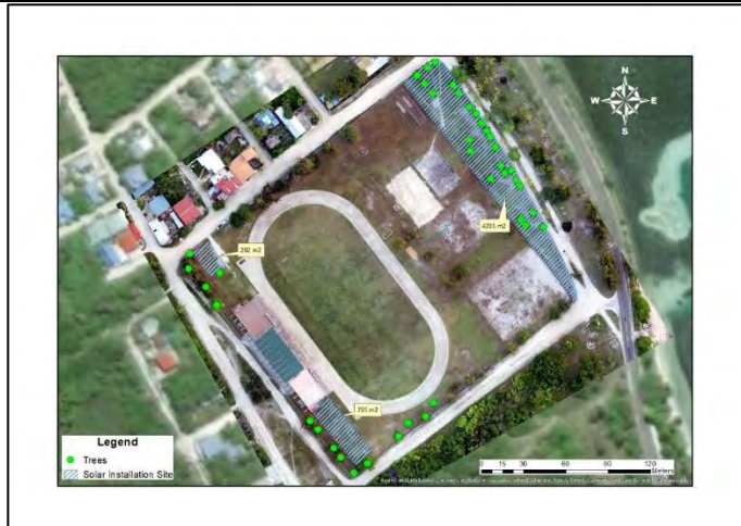
FIGURE 3 PV INSTALLATION AREA AT ADDU FOOTBALL STADIUM
