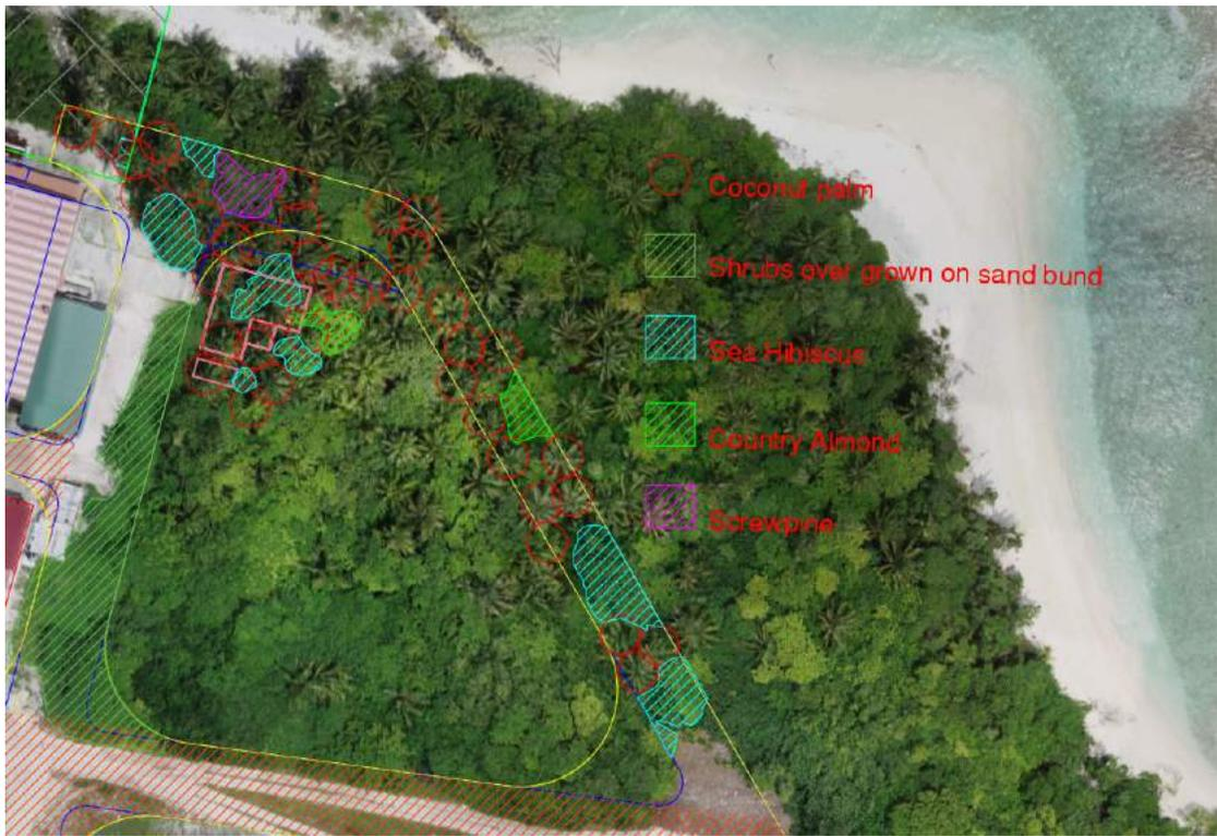
Figure 17. Areas which require vegetation clearance to develop the plots (red) and roads (yellow) as per the proposed master plan
