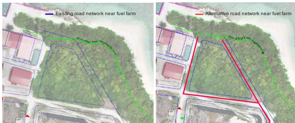
**Figure 25. Proposed road network extensions (blue highlight) and alternate road network extensions (red) for RWMF at Vandhoo, thick green line shows 20m offset from vegetation line (EPZ extent)**
