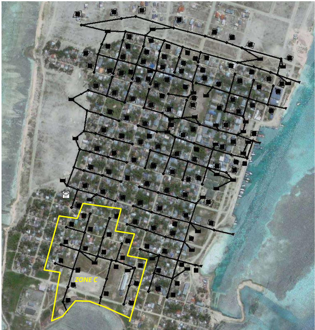
Figure 6.13 -: Location of Zone “C” with in the Thinadhoo drainage network of SWMM
