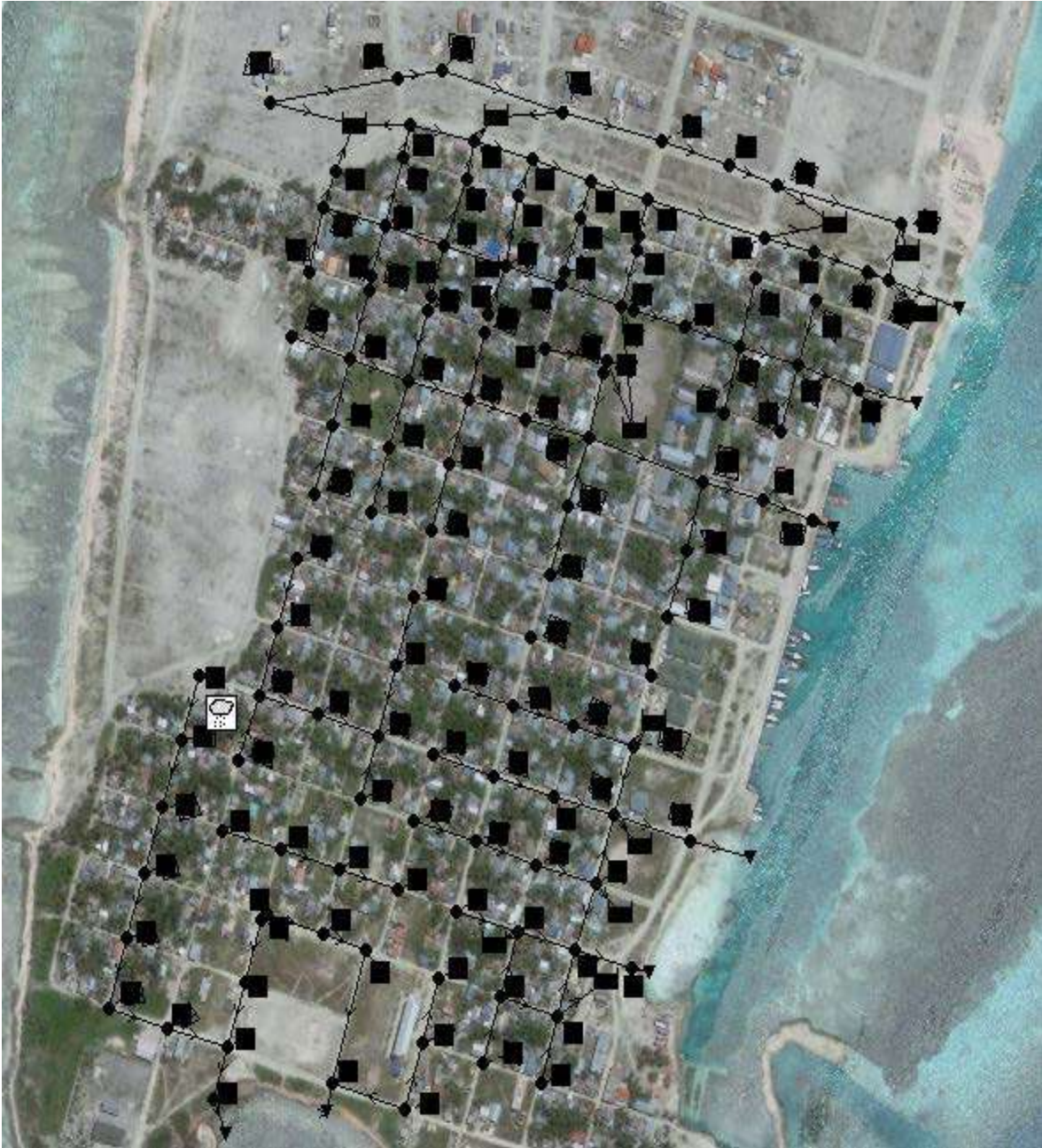
Figure 6.1 SWMM model set up for G Dh Thinadhoo Island
