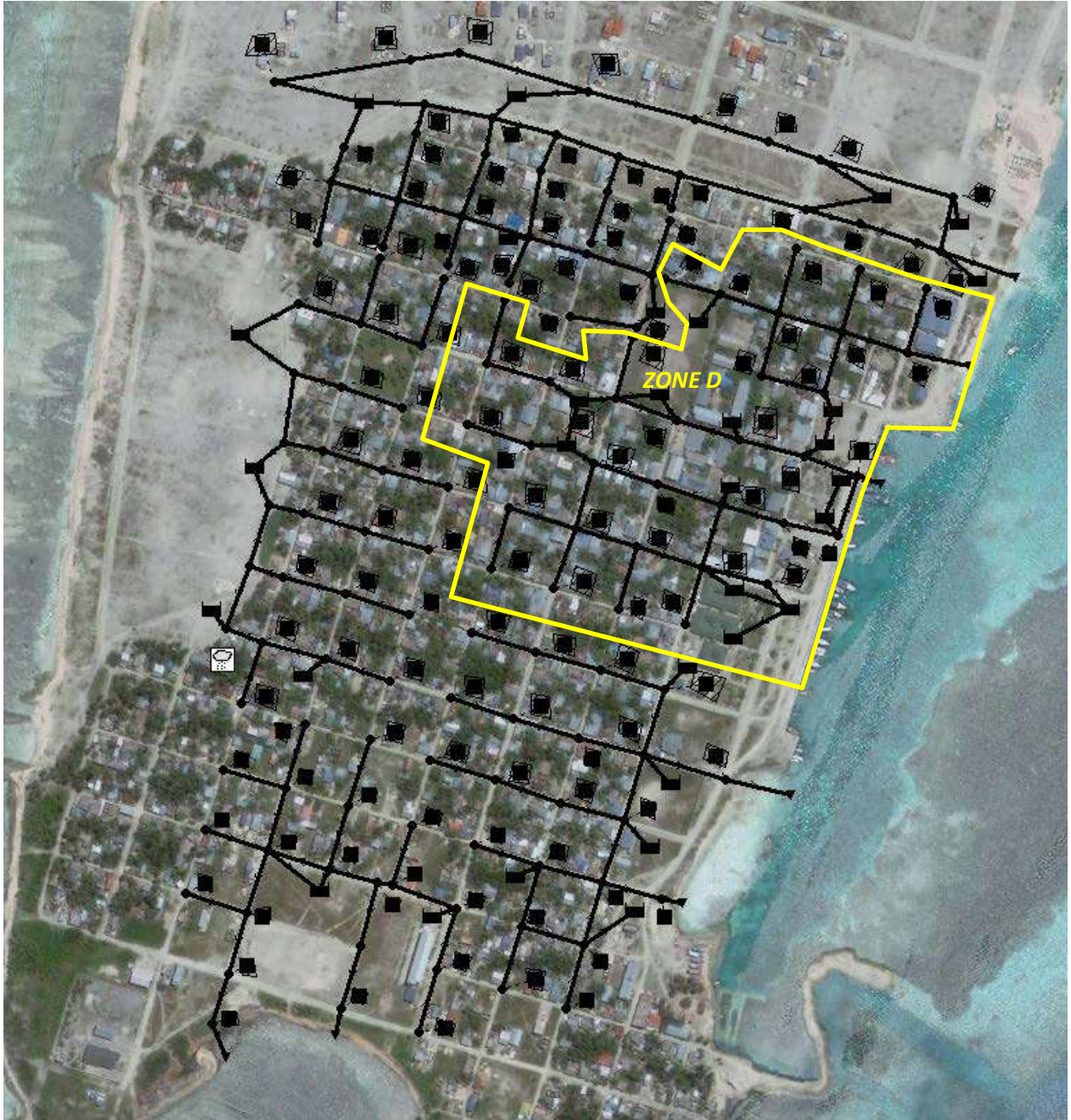
Figure 6.16 -: Location of Zone “D” with in the G Dh Thinadhoo drainage network of SWMM model
