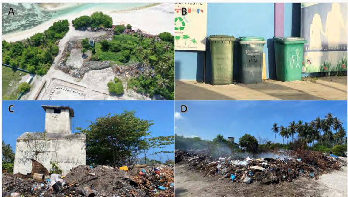
Figure 2: Photos from Guraidhoo. (a) drone photo of current waste dump site, (b) bins at a public collection point, (c) waste burning house (community made incinerator) and (d) open burning at waste dump site
