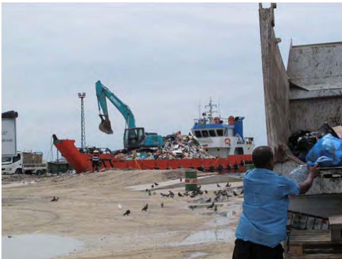
Figure 14: Existing Situation. The transfer of waste from delivery trucks to barges is time consuming and inefficient, and significant volumes of waste are lost to the
