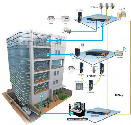
Figure 23: Smart sensors network and centralized smart building energy management system
