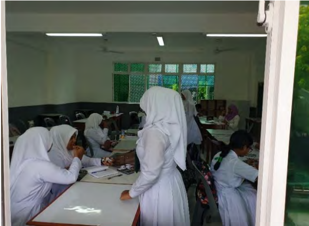
Figure 101– Image showing low daylight levels in classrooms located near the external window
