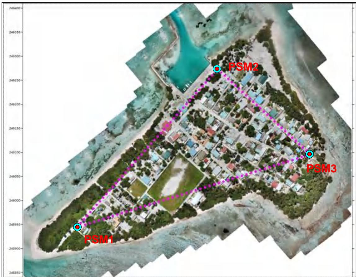
Figure 1-7: Example of spacing of PSMs
