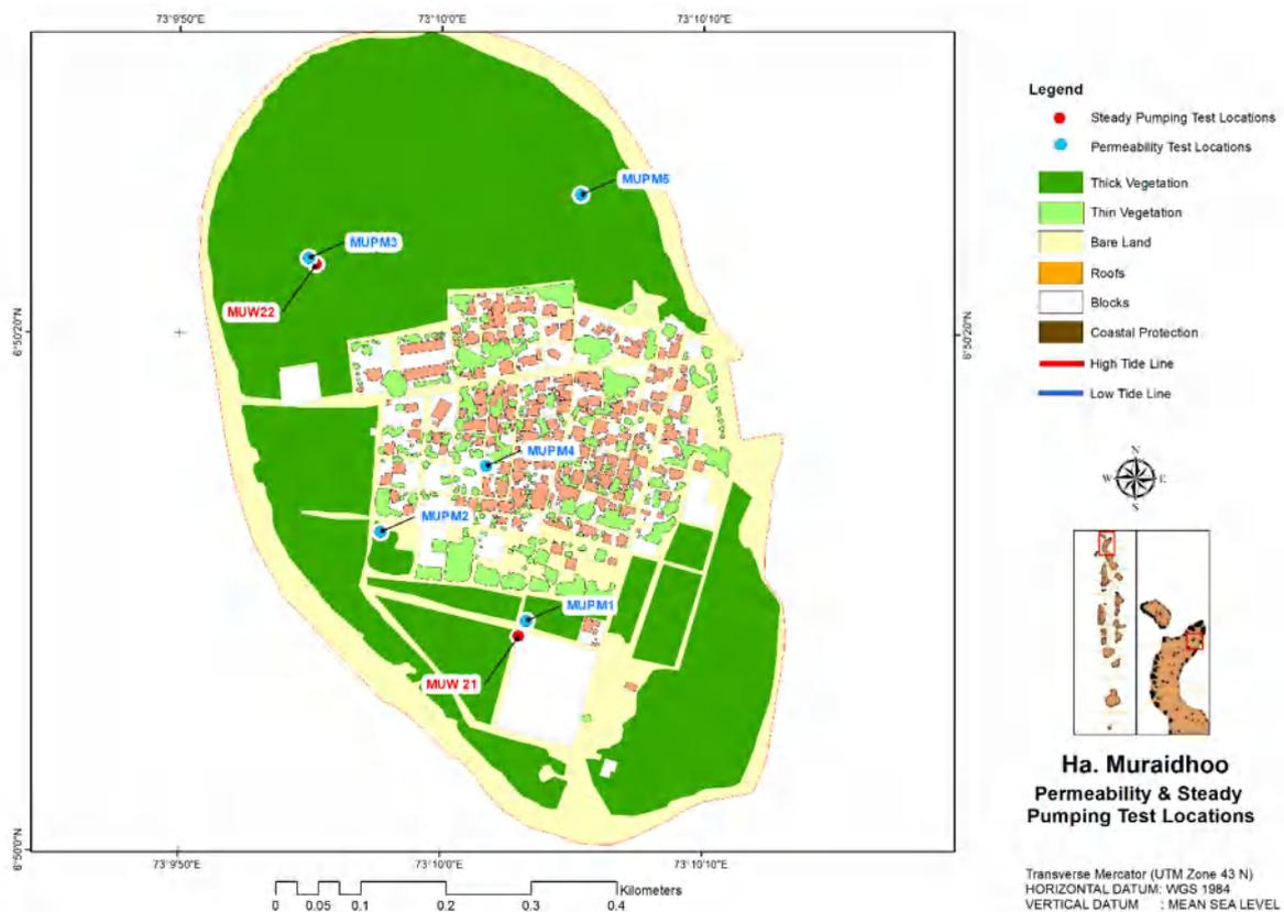
Figure 5-21: Locations of permeability and steady pumping tests in Muraidhoo Island
