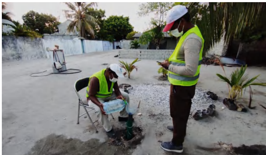
Figure 1-10: Methodology for Constant Head Gravity Permeability Tests
