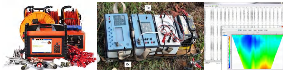
Figure 1-4: Electrical Resistivity (ER) equipment used for the field pilot tests (Sources: Left - ABEM Terrameter LS 2 - User Manual, 2017/ Center, Right - Siqueira Neto & Elis)
