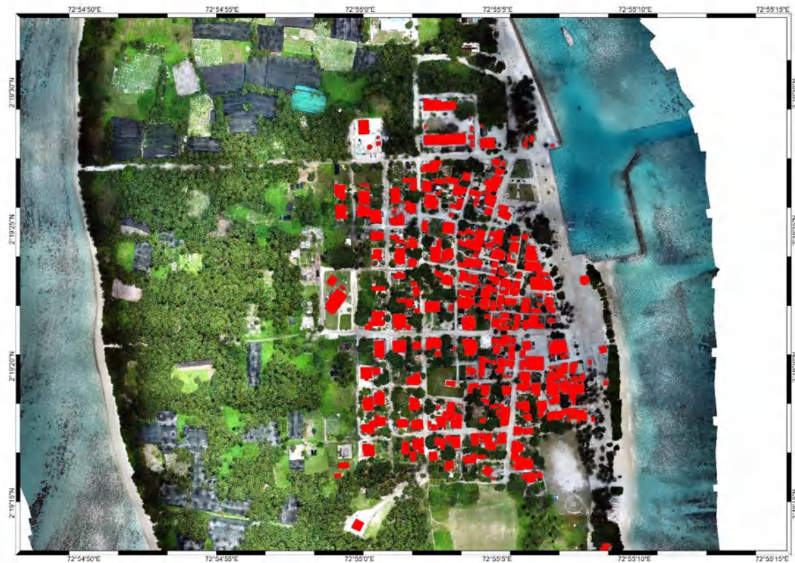
Figure 1-9: Calculation of Roof Cover in an island using UAV survey in the Maldives
