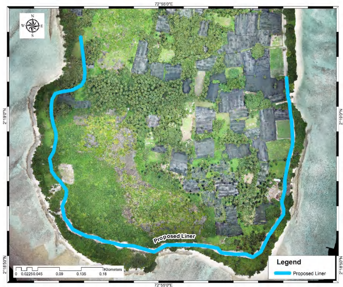
Figure 4-11: Proposed area for the installation of clay liner parallel to the road
