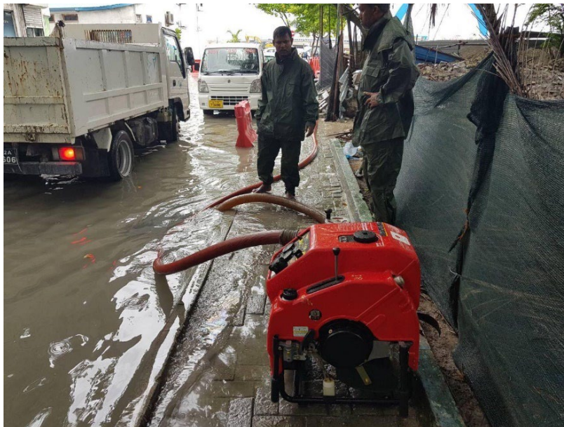
Figure 2.1: Mobile pumps are used occasionally to drain stormwater from the streets of Male' city after a heavy rain shower. (Source: psmnews.mv/en/40417)
