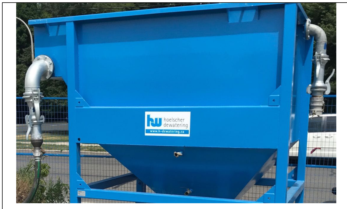
Figure 4.6: Silt traps acting as filters that can be used to clean water before discharging (Source: drainagepipe.co.uk/soakaways-and-membranes/what-is-a-silt-trap-and-why-should-i-have-one/ )
