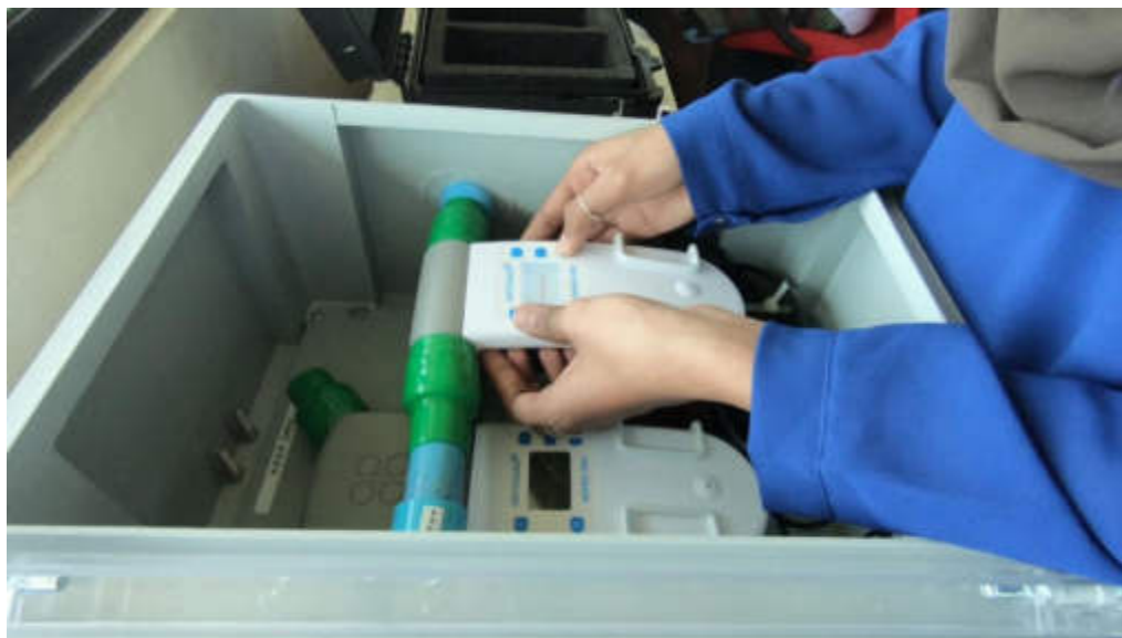
Figure 1: Air Quality monitoring station with two Aeroqual Series 500 monitors
