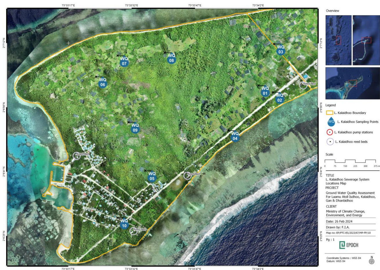
Figure 6.3: L. Kalaidhoo Sewerage System Locations
