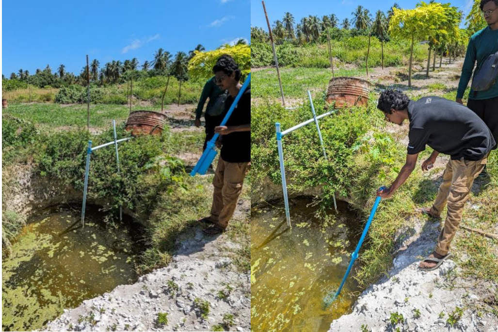
Figure 4.2: Collecting groundwater samples directly from well using custom-made bailer
