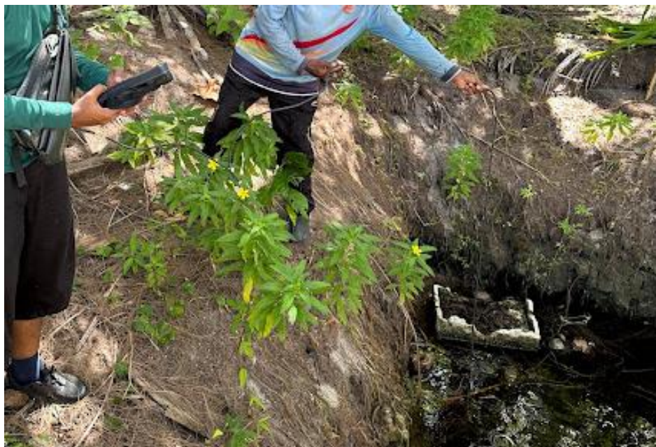
Figure 4.1. Groundwater sampling by dipping YSI ProDSS probes directly into the well
