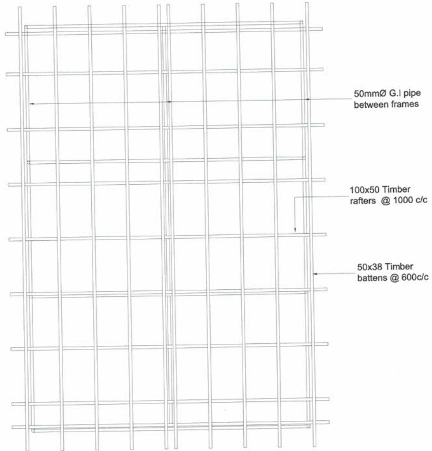
ROOF FRAMING PLAN FORMER PRESCHOOL SITE
