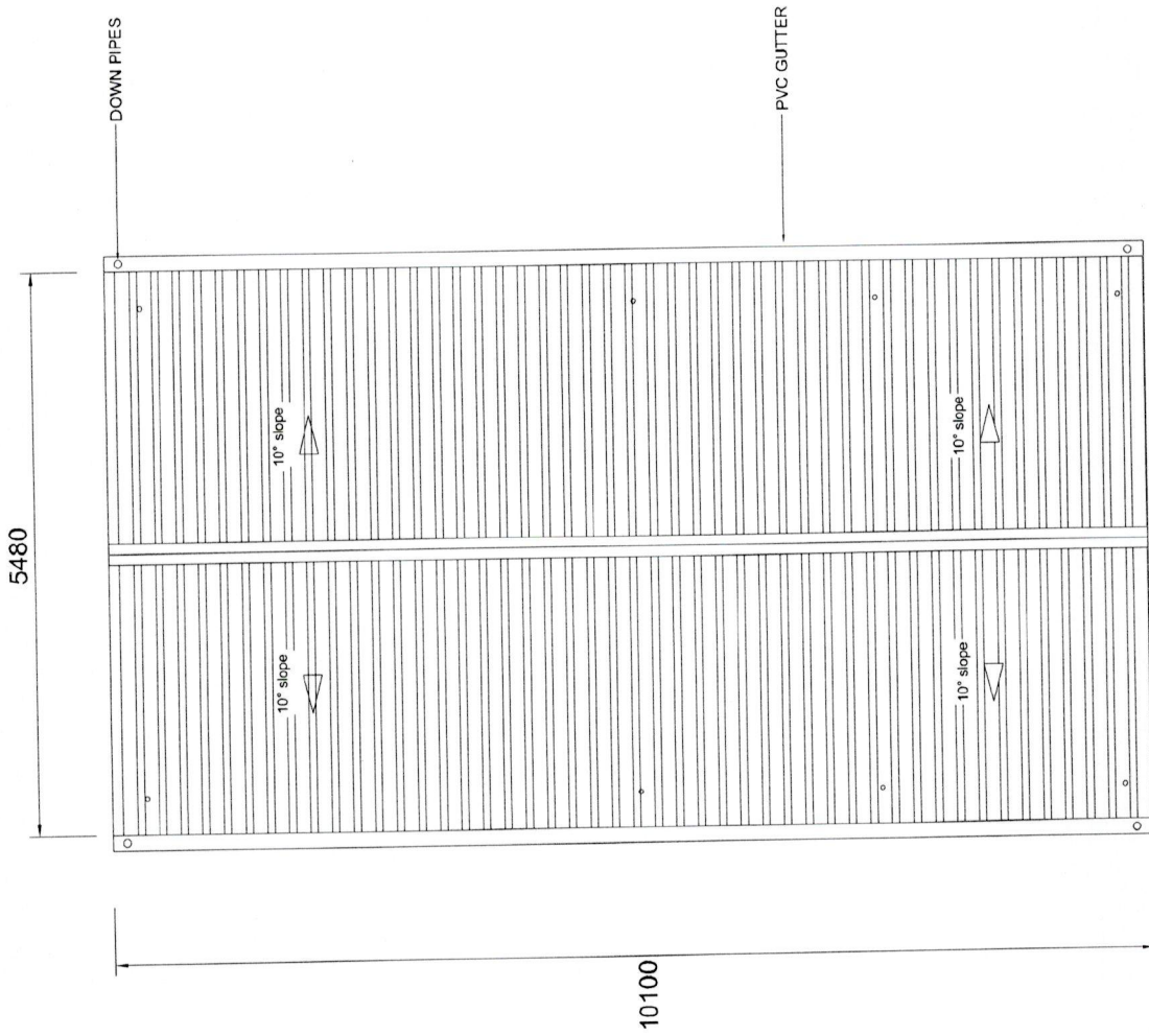
ROOF PLAN OVER WATER TANKS TUTHIMAAEE SITE
