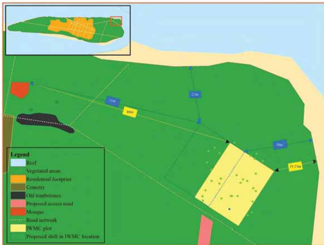
Figure 18: Proposed adjustment of IWMC site to increase distance between site and vegetation line
