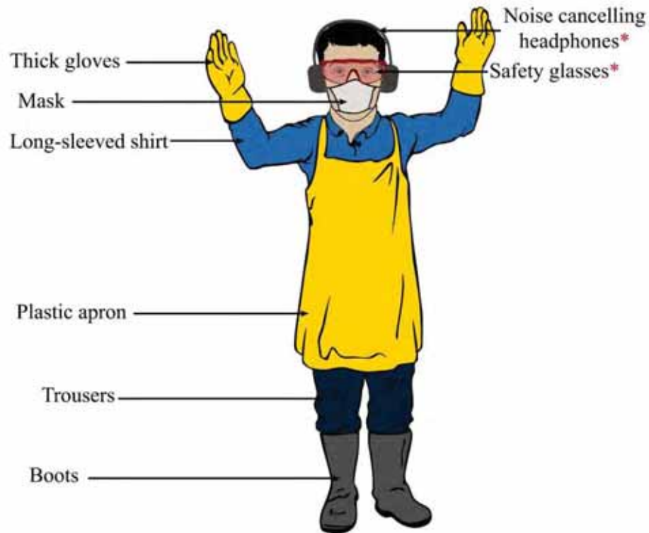
Figure 19: Recommended protective clothing for waste management employees. Adapted From: Ministry of Health, Thailand. Bangkok, 1995. *noise cancelling headphones and safety glasses during use of machinery
