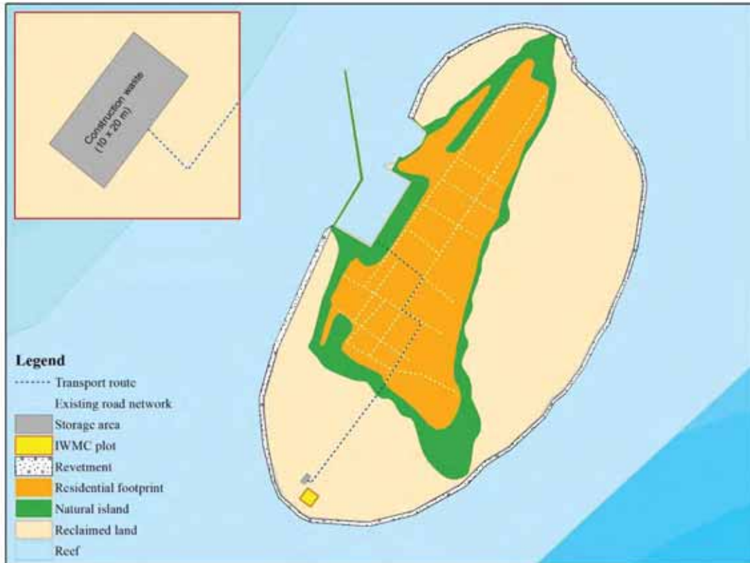
Figure 7: Transportation route and storage area
