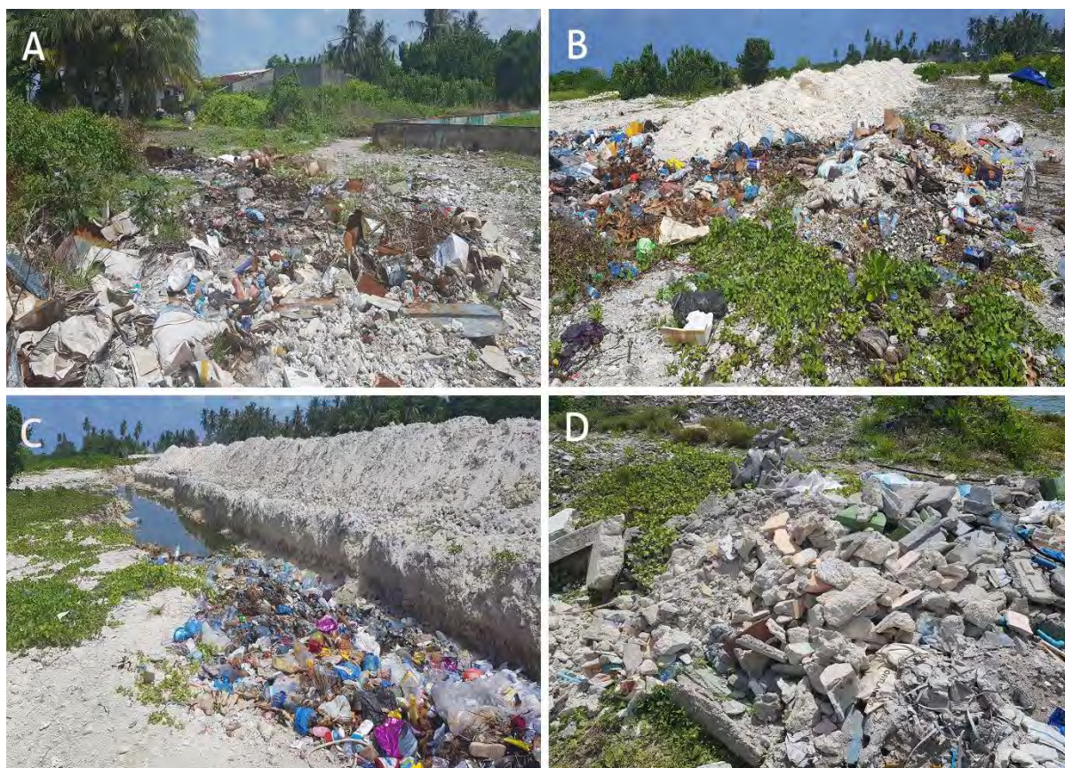
Figure 5: Current state of waste disposal in the island. (A) Collection of waste near the dumpsite (B) and (C) Trench dug at the islands existing dumpsite (D) Construction waste dumped near the islands harbour.
