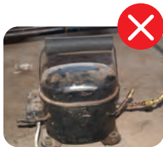
FIGURE 8: COMPRESSORS MUST NOT BE USED FOR VACUUMING
