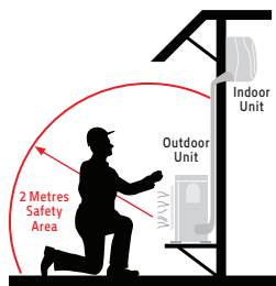
FIGURE 5: TEMPORARY FLAMMABLE ZONE
