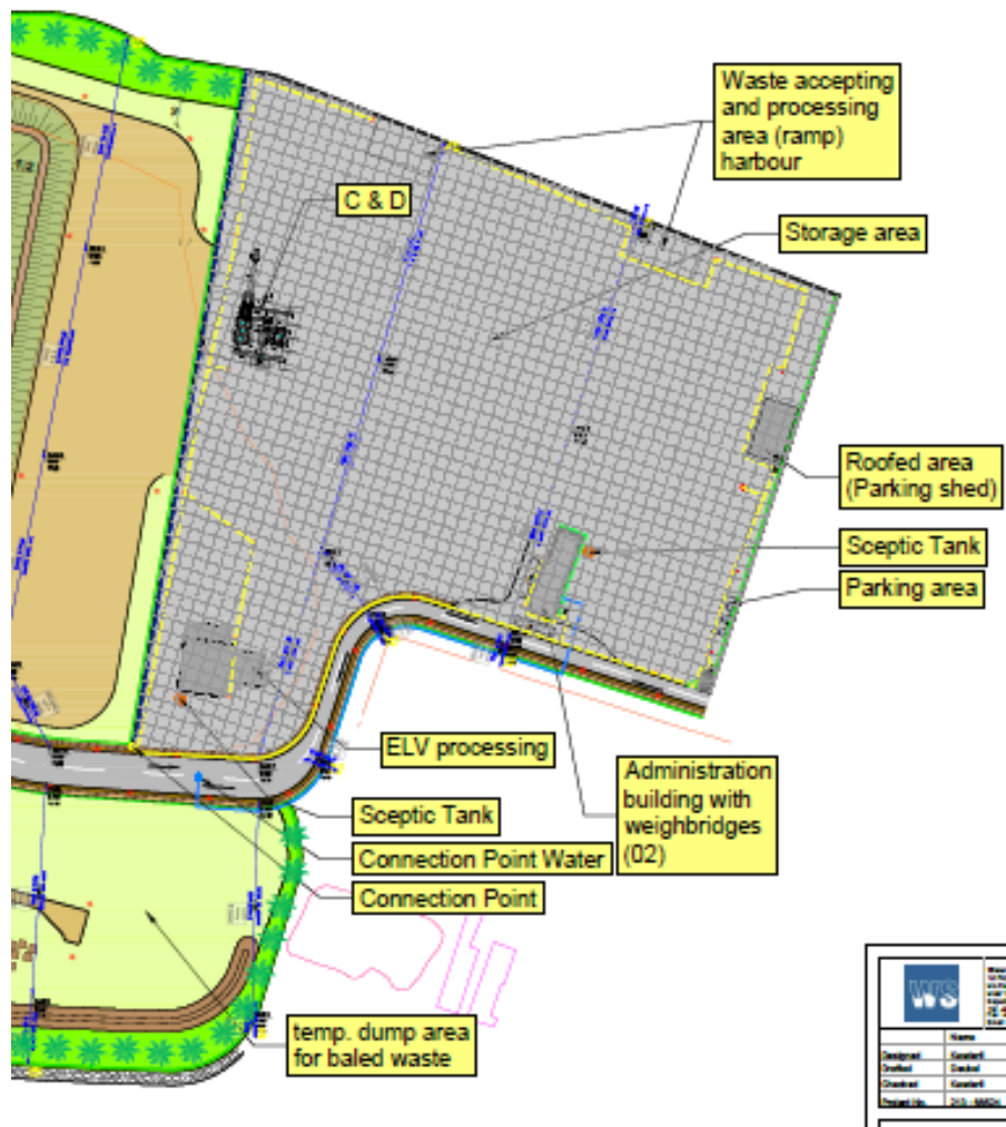
Figure 3: Proposed layout of the eastern end of the RWMF showing locations of the proposed facilities
