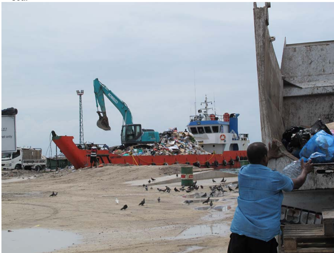
Figure 13: Existing Situation. The transfer of waste from delivery trucks to barges is time consuming and inefficient, and significant volumes of waste are lost to the sea.
