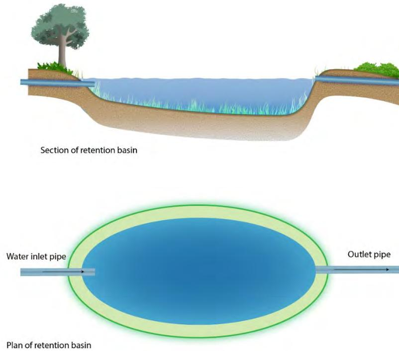
Figure 2.19: Typical details of a retention basin
