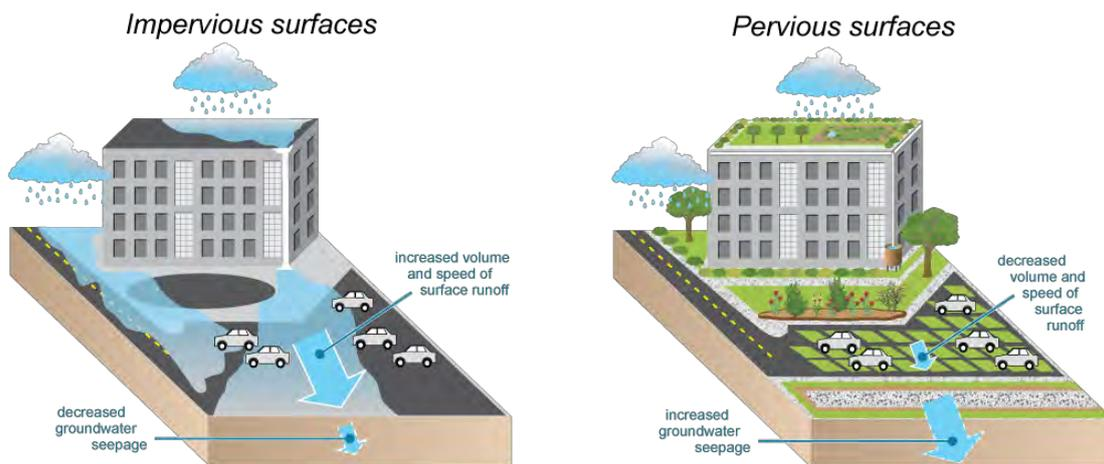
Figure 5: A conceptual diagram showing the difference between pervious and impervious surfaces (Adapted from Source: [umces.edu/ian/library/impervious-versus-pervious-surfaces](http://umces.edu/ian/library/impervious-versus-pervious-surfaces))
