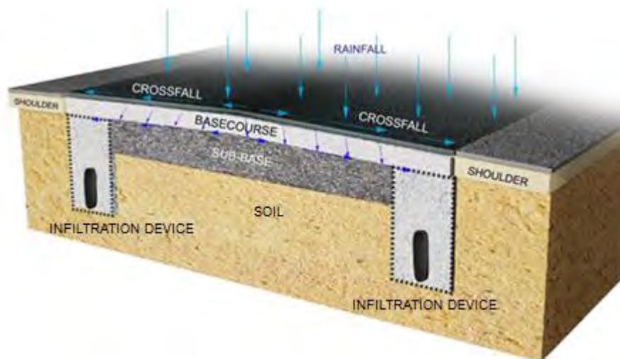
*Figure 2.11: Schematic of a cross-section through a road which shows the concept of road drainage using infiltration devices constructed on either side of the road. (Adapted from Source: geosynthetica.com)*
