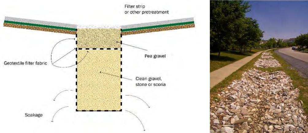
Figure 2.20: Cross-section through an infiltration trench (left). An infiltration trench constructed on the road side(right) (Source: sswm.info)
