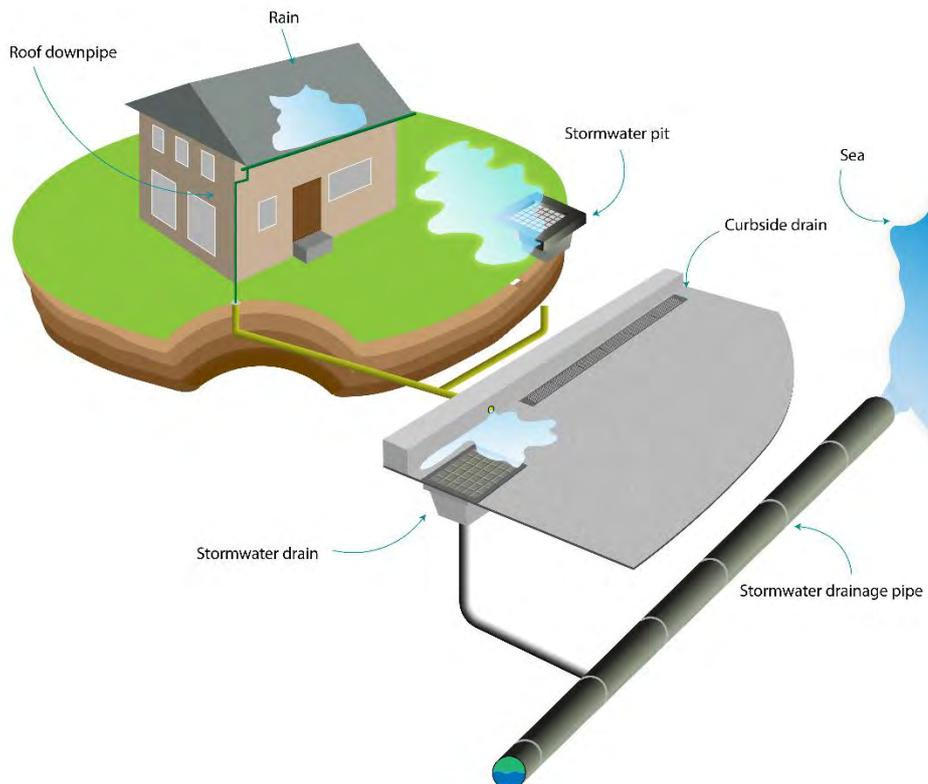
*Figure 2.6: Schematic perspective of a separated stormwater drainage system showing the basic processes of the system (collection, transportation and discharging)*
