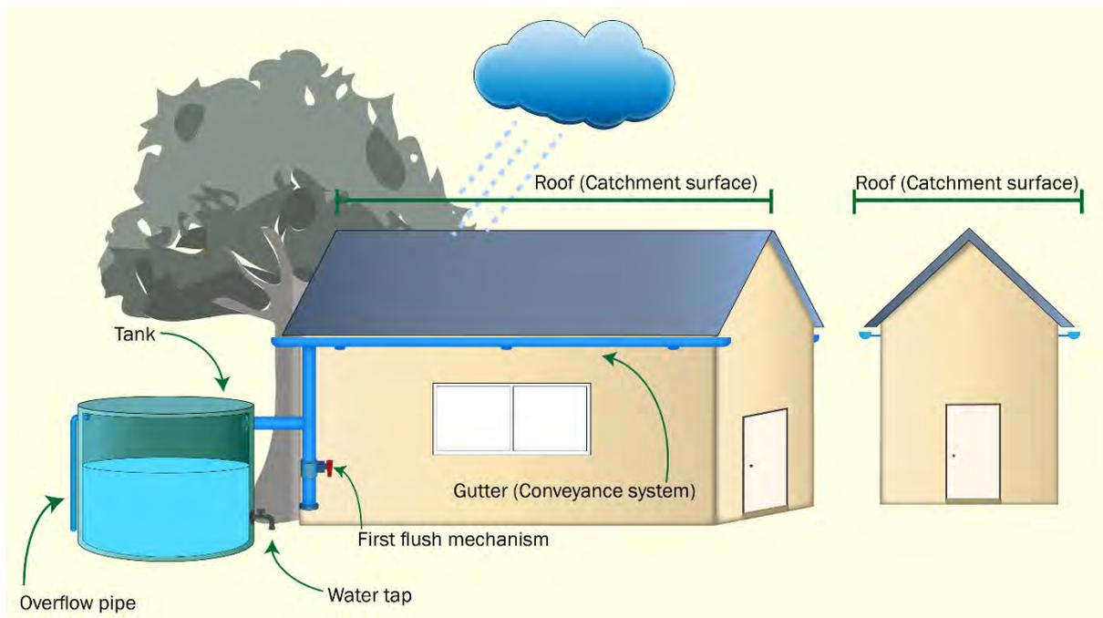
*Figure 1.1: Building roofs are used as rainwater catchment surfaces*
