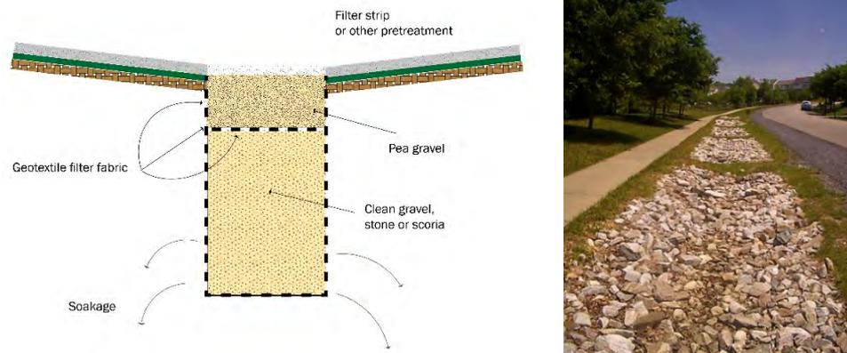
Figure 1.8: Cross-section through an infiltration trench (left). Example photo of an infiltration trench constructed on the road side(right) (Adapted from Source: [sswm.info](http://sswm.info))
