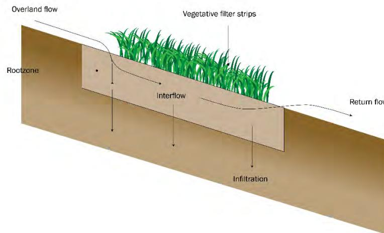
Figure 1.11: Cross-section through a typical grassed filter strip
