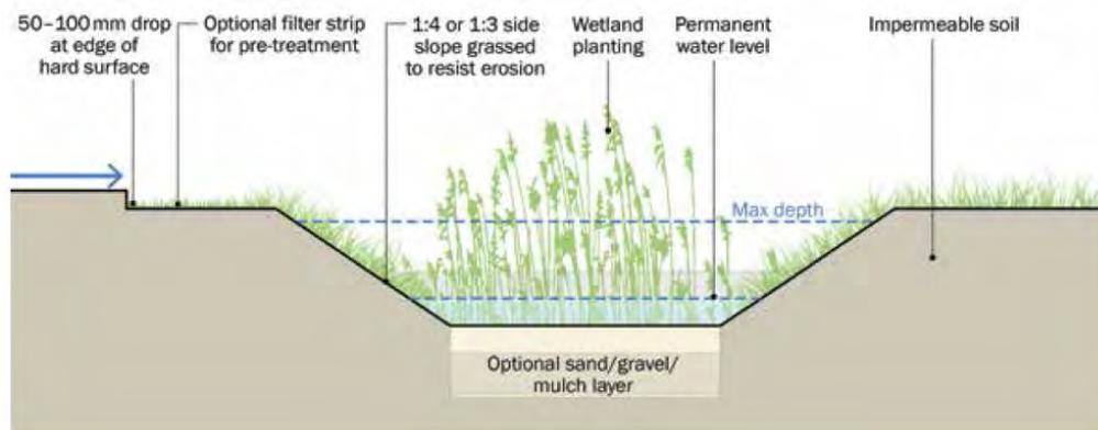
Figure 2.16: Typical section through a swale (CIRIA, 2015, p. 315)
